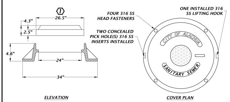
FRAME AND COVER SECTION WITH COVER SHOWN REMOVED FROM FRAME (ALL DIMENSIONS ARE NOMINAL)
